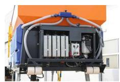
the eStratos is significantly quieter. In addition, the safe 48 V DC system can be maintained without special training or safety measures.
