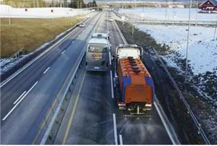
The Straliq is specially designed for spraying brine from large carrier vehicles using the three-lane spraying technique, which enables fast and efficient de-icing. The Straliq has a capacity of 7,500 -15,000 litres, which means that very large areas can be de-iced in one operation, while the high quality polyethylene tanks are suitable for all de-icing agents. Significant savings in consumption of spraying materials can be achieved, especially down to -6° C.
