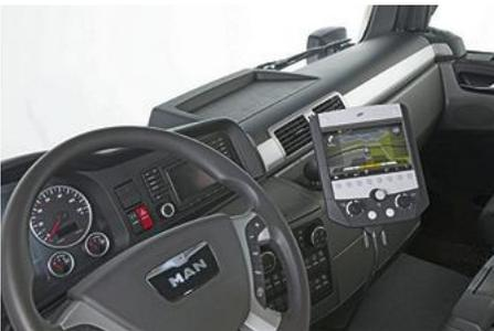
The Straliq is operated from the driver's cab using the highly effective ES control panel. Easy-grip click-turn knobs and illuminated push buttons ensure that the driver can concentrate fully on the traffic and road conditions. In conjunction with the **ThermoLogic** and **AutoLogic** systems, the Straliq becomes even more efficient and resource-saving.
