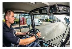
All functions of the washing unit are controlled via the door control panel with various joysticks and push buttons. The most important information is visible at a glance on the colour display in the roof console. In addition, a mechanic can make machine-specific settings in the display. With the aid of the onboard diagnosis system, any faults can be localised quickly and efficiently.
