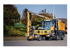
The **Cleango 500 SKR** has a fresh water volume of 685 I and thus enables long working hours. Optionally, the water volume can be expanded via additional tanks.
