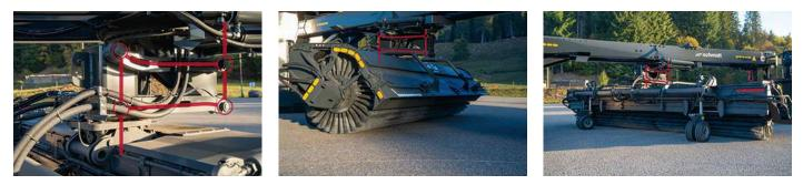
The twin castors offer very quiet, vibration-free and smooth sweeping performance, while level snow ejection and the cleanest fine clearing ensure maximum safety. This is achieved thanks to aerodynamic spoiler guidance, automatic spoiler adjustment and wear-dependent brush speed adjustment. This permits the jet sweeper to deliver a specific fine clearing result, while the robust design offers both optimum operational capability and maximum safety.
