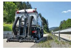
lision protection. The rear suction unit is not dependent on the type of truck and its operation is fully integrated into the ES control panel, enabling simple and easy control whilst driving.
