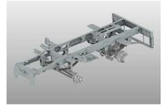
ving even in bad road and weather conditions. The MFH 550 has the highest payload in its class - up to 6,600 kg thanks to robust suspension, high axle loads and twin tyres on the rear axle.
