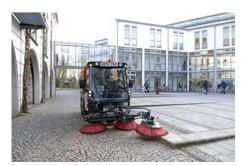
Optional lowerable, self-levelling running gear simplifies driving in multi-storey car parks and low entrances as the chassis can be lowered by 70mm at the push of a button.
