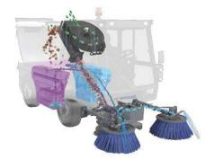
The 2-brush system with independently controlled circular brushes guarantees absolute mobility in every sweeping situation. Two stable brush arms with integrated buffers allow sweeping widths of up to 2,900 mm.
