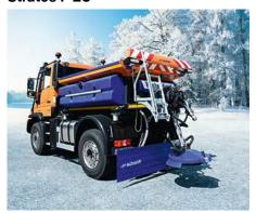
The Stratos F25 is a flat silo spreader with a hopper capacity of  $2.5 \, \text{m}^3$ .
