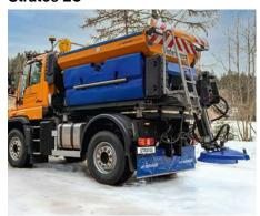
The Stratos 25 is a silo spreader with a hopper capacity of 2.5 m<sup>3</sup>.
