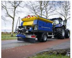
The Stratos A50K is a trailer spreader with a hopper capacity of 5  $m^3.$
