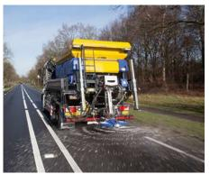
The Stratos 50 is a mounted spreader with a hopper capacity of 5  $m^3$ .
