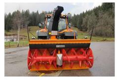
The cutter drums with the double-threaded open cutting spirals guarantee optimum snow transport to the impeller due to the cutting blades that become wider towards the inside. The outside mounted cutter drums ensure a stable hold and, in combination with the attached side cutters, very good steerability of the carrier vehicle is ensured. The cutter drums are driven via a robust central mounted bevel gear and are protected by self-readjusting clutches.
